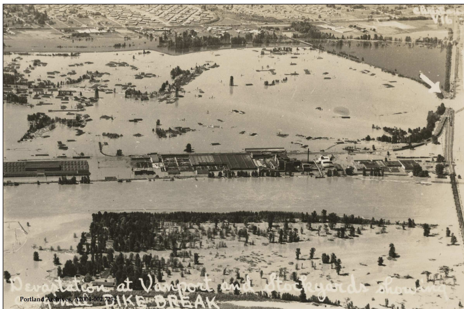
Figure 9. Aerial view of the Vanport flood. Arrow at upper right indicates the location of the railroad bank breach. Image is from above Hayden Island in the Columbia River, looking south towards Kenton. The dark stretch across the center of the image is the infrastructure of the Portland stockyards, also under water. Portland City Archives
